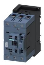
power contactor, AC-3e/AC-3, 95 A, 45 kW / 400 V, 3-pole, 24 V DC, 0.8-1.2\* Us, with integrated varistor, auxiliary contacts: 1 NO + 1 NC, integrated varistor, main circuit: screw terminal, control and auxiliary circuit: spring-loaded terminal, suitable for PLC outputs
