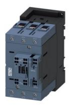
power contactor, AC-3e/AC-3, 95 A, 45 kW / 400 V, 3-pole, 20-33 V AC/DC, 50/60 Hz, with integrated varistor, auxiliary contacts: 1 NO + 1 NC, main circuit: screw terminal, control and auxiliary circuit: spring-loaded terminal, communication-capable
