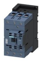
power contactor, AC-3e/AC-3, 95 A, 45 kW / 400 V, 3-pole, 175-280 V AC/DC, 50/60 Hz, with integrated varistor, auxiliary contacts: 1 NO + 1 NC, main circuit: screw terminal, control and auxiliary circuit: spring-loaded terminal
