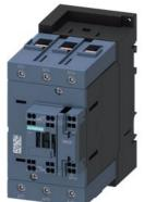
traction contactor, AC-3e/AC-3, 95 A, 45 kW / 400 V, 3-pole, 24 V DC, 0.7-1.25\* Us, electronic drive, with integrated varistor, auxiliary contacts: 1 NO + 1 NC, main circuit: screw terminal, control and auxiliary circuit: springloaded terminal
