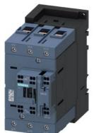
traction contactor, AC-3e/AC-3, 95 A, 45 kW / 400 V, 3-pole, 110 V DC, 0.7-1.25\* Us, electronic drive, with integrated varistor, auxiliary contacts: 1 NO + 1 NC, main circuit: screw terminal, control and auxiliary circuit: spring-loaded terminal
