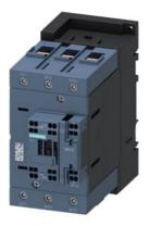
traction contactor, AC-3e/AC-3, 95 A, 45 kW / 400 V, 3-pole, 72 V DC, 0.7-1.25\* Us, electronic drive, with integrated varistor, auxiliary contacts: 1 NO + 1 NC, main circuit: screw terminal, control and auxiliary circuit: spring-loaded terminal
