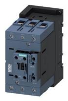
power contactor, AC-3e/AC-3, 110 A, 55 kW / 400 V, 3-pole, 175-280 V AC/DC, 50/60 Hz, with integrated varistor, auxiliary contacts: 1 NO + 1 NC, screw terminal
