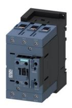
traction contactor, AC-3e/AC-3, 110 A, 55 kW / 400 V, 3-pole, 24 V DC, 0.7-1.25 $^{\star}$  Us, electronic drive, with integrated varistor, auxiliary contacts: 1 NO + 1 NC, screw terminal
