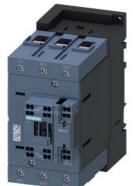
power contactor, AC-3e/AC-3, 110 A, 55 kW / 400 V, 3-pole, 175-280 V AC/DC, 50/60 Hz, with integrated varistor, auxiliary contacts: 1 NO + 1 NC, main circuit: screw terminal, control and auxiliary circuit: spring-loaded terminal
