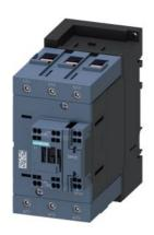
traction contactor, AC-3e/AC-3, 110 A, 55 kW / 400 V, 3-pole, 110 V DC, 0.7-1.25\* Us, electronic drive, with integrated varistor, auxiliary contacts: 1 NO + 1 NC, main circuit: screw terminal, control and auxiliary circuit: spring-loaded terminal
