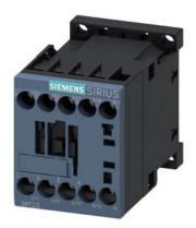
Contactor, AC-1, 18 A/400 V/40  $^{\circ}\text{C},$  S00, 4-pole, 110 V AC, 50/60 Hz, screw terminal
