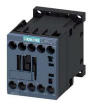
contactor AC-1, 22 A, 400 V / 40 °C, 4-pole, 12 V DC, screw terminal, size: S00  $\,$
