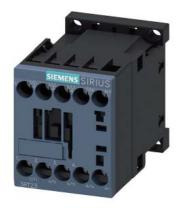
contactor AC-1, 22 A, 400 V / 40  $^{\circ}\text{C},$  4-pole, 125 V DC, screw terminal, size: S00
