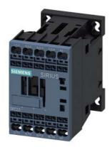
contactor AC-1, 22 A, 400 V / 40  $^{\circ}$ C, 4-pole, 110 V AC, 50 Hz / 120 V, 60 Hz, spring-loaded terminal, size: S00
