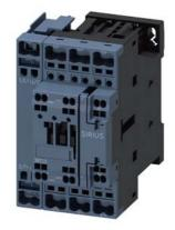
contactor AC-1, 35 A, 400 V / 40 °C, 4-pole, 110 V AC, 50 Hz / 120 V, 60 Hz, auxiliary contacts: 1 NO + 1 NC, spring-loaded terminal, size: S0
