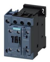
Contactor, AC-1, 40 A/400 V/40  $^{\circ}$ C, S0, 4-pole, 110 V AC/50 Hz, 120 V/60 Hz, 1 NO+1 NC, screw terminal
