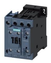
contactor AC-1, 40 A, 400 V / 40 °C, 4-pole, 220 V DC, auxiliary contacts: 1 NO + 1 NC, screw terminal, size: S0
