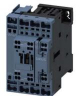
contactor AC-1, 40 A, 400 V / 40 °C, 4-pole, 110 V AC, 50 Hz / 120 V, 60 Hz, auxiliary contacts: 1 NO + 1 NC, spring-loaded terminal, size: S0
