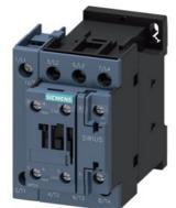
contactor AC-1, 50 A, 400 V / 40 °C, 4-pole, 230 V AC, 50/60 Hz, auxiliary contacts: 1 NO + 1 NC, screw terminal, size: S0
