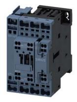
contactor AC-1, 50 A, 400 V / 40 °C, 4-pole, 110 V AC, 50 Hz / 120 V, 60 Hz, auxiliary contacts: 1 NO + 1 NC, spring-loaded terminal, size: S0
