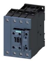
contactor AC-1, 110 A, 400 V / 40  $^{\circ}$ C, 4-pole, 230 V AC, 50 Hz, auxiliary contacts: 1 NO + 1 NC, screw terminal
