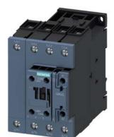
contactor AC-1, 110 A, 400 V / 40 °C, 4-pole, 20-33 V AC/DC, 50/60 Hz, with integrated varistor, auxiliary contacts: 1 NO + 1 NC, screw terminal
