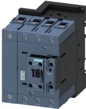
Schütz, AC-1, 140 A/400 V/40 °C, S3, 4-polig, AC/DC 20-33V, 1S+1Ö, Schraubanschluss
