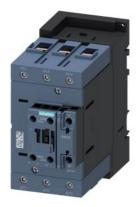
contactor AC-1, 140 A, 690 V / 40  $^{\circ}$ C, 3-pole, 24 V AC, 50/60 Hz, auxiliary contacts: 1 NO + 1 NC, main circuit: box terminal, control and auxiliary circuit: screw terminal
