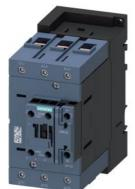
contactor AC-1, 140 A, 690 V / 40 °C, 3-pole, 175-280 V AC/DC, 50/60 Hz, with integrated varistor, auxiliary contacts: 1 NO + 1 NC, main circuit: box terminal, control and auxiliary circuit: screw terminal
