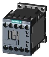
Power contactor, AC-3 9 A, 4 kW / 400 V 2 NO + 2 NC 208 V AC, 50/60 Hz 4-pole Size S00 screw terminals
