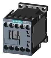
Contactor, 2NO + 2NC, AC-3, 5.5 kW, 110 V AC, 50 Hz, 120 V, 60Hz, 4-pole, 2NO + 2NC, Size S00, Screw terminal
