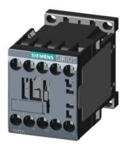
power contactor, AC-3e/AC-3, 16 A, 7.5 kW / 400 V, 4-pole, main contacts: 2 NO + 2 NC, 220 V AC, 50 Hz / 240 V, 60 Hz, screw terminal
