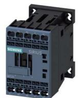
Contactor, 2NO + 2NC, AC-3, 7.5 kW, 110 V AC, 50 Hz, 120 V, 60Hz, 4-pole, 2NO + 2NC, Size S00, Spring-type terminal
