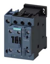
power contactor, AC-3e/AC-3, 25 A, 11 kW / 400 V, 4-pole, 230 V AC, 50 Hz, main contacts: 2 NO + 2 NC, auxiliary contacts: 1 NO + 1 NC, screw terminal
