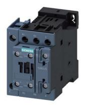
power contactor, AC-3e/AC-3, 25 A, 11 kW / 400 V, 4-pole, main contacts: 2 NO + 2 NC, 125 V DC, auxiliary contacts: 1 NO + 1 NC, screw terminal
