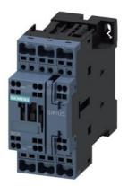
power contactor, AC-3e/AC-3, 25 A, 11 kW / 400 V, 4-pole, 24 V DC, main contacts: 2 NO + 2 NC, auxiliary contacts: 1 NO + 1 NC, spring-loaded terminal
