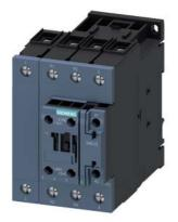
power contactor, AC-3e/AC-3, 40 A, 18.5 kW / 400 V, 4-pole, 110 V AC, 50 Hz, main contacts: 2 NO + 2 NC, auxiliary contacts: 1 NO + 1 NC, screw terminal
