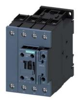
power contactor, AC-3e/AC-3, 40 A, 18.5 kW / 400 V, 4-pole, 230 V AC, 50/60 Hz, main contacts: 2 NO + 2 NC, auxiliary contacts: 1 NO + 1 NC, screw terminal
