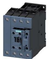
power contactor, AC-3e/AC-3, 51 A, 22 kW / 400 V, 4-pole, 20-33 V AC/DC, 50/60 Hz, with integrated varistor, main contacts: 2 NO + 2 NC, auxiliary contacts: 1 NO + 1 NC, screw terminal
