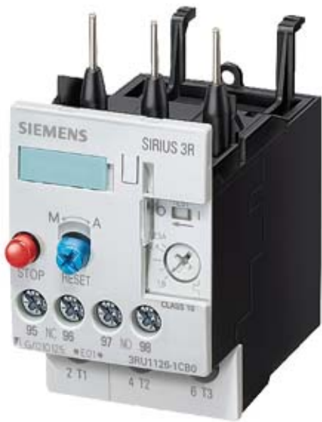
OVERLOAD RELAY, 4.5...6.3 A, 1NO+1NC, SIZE S0, CLASS 10, FOR CONTACTOR MOUNTING
