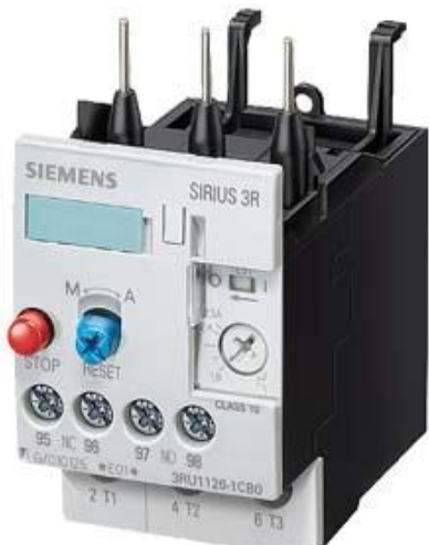
OVERLOAD RELAY, 5.5...8 A, 1NO+1NC, SIZE S0, CLASS 10, FOR CONTACTOR MOUNTING
