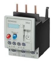
Overload relay 14...20 A For motor protection Size S2, Class 10 Contactor mounting Main circuit: Screw terminal Auxiliary circuit: Screw terminal Manual-Automatic-Reset !!! Phased-out product !!! Successor is SIRIUS 3RU2 Preferred successor type is >>3RU2136-4BB0<<
