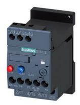
Overload relay 0.11...0.16 A Thermal For motor protection Size S00, Class 10 Stand-alone installation Main circuit: Screw Auxiliary circuit: Screw Manual-Automatic-Reset
