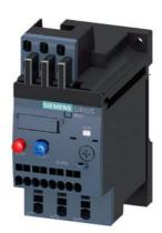
Overload relay 0.14...0.20 A Thermal For motor protection Size S00, Class 10 Stand-alone installation Main circuit: Spring-type terminal Auxiliary circuit: spring-type terminal Manual-Automatic-Reset
