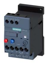
Overload relay 0.90...1.25 A Thermal For motor protection Size S00, Class 10 Stand-alone installation Main circuit: Screw Auxiliary circuit: Screw Manual-Automatic-Reset
