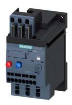
Overload relay 0.90...1.25 A Thermal For motor protection Size S00, Class 10 Stand-alone installation Main circuit: Spring-type terminal Auxiliary circuit: spring-type terminal Manual-Automatic-Reset
