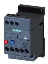
Overload relay 4.5...6.3 A Thermal For motor protection Size S00, Class 10 Stand-alone installation Main circuit: Screw Auxiliary circuit: Screw Manual-Automatic-Reset
