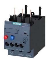
Overload relay 2.2...3.2 A Thermal For motor protection Size S0, Class 10 Contactor mounting Main circuit: Screw Auxiliary circuit: Screw Manual-Automatic-Reset
