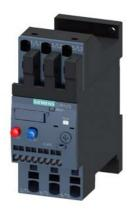
Overload relay 14...20 A Thermal For motor protection Size S0, Class 10 Stand-alone installation Main circuit: Spring-type terminal Auxiliary circuit: spring-type terminal Manual-Automatic-Reset
