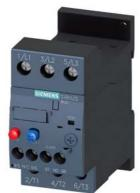
Overload relay 17...22 A Thermal For motor protection Size S0, Class 10 Stand-alone installation Main circuit: Screw Auxiliary circuit: Screw Manual-Automatic-Reset
