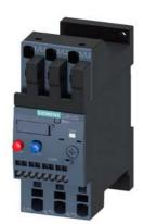
Overload relay 17...22 A Thermal For motor protection Size S0, Class 10 Stand-alone installation Main circuit: Spring-type terminal Auxiliary circuit: spring-type terminal Manual-Automatic-Reset
