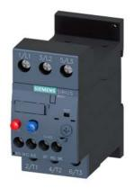
Overload relay 20...25 A Thermal For motor protection Size S0, Class 10 Stand-alone installation Main circuit: Screw Auxiliary circuit: Screw Manual-Automatic-Reset
