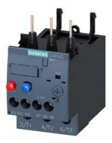
Overload relay 23...28 A Thermal For motor protection Size S0, Class 10 Contactor mounting Main circuit: Screw Auxiliary circuit: Screw Manual-Automatic-Reset
