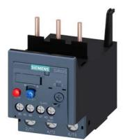
Overload relay 14...20 A Thermal For motor protection Size S2, Class 10 Contactor mounting Main circuit: Screw Auxiliary circuit: Screw Manual-Automatic-Reset
